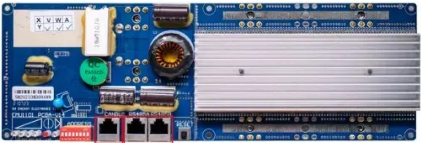
RS485 Communication between battery and inverters Baud rate:9600bps
